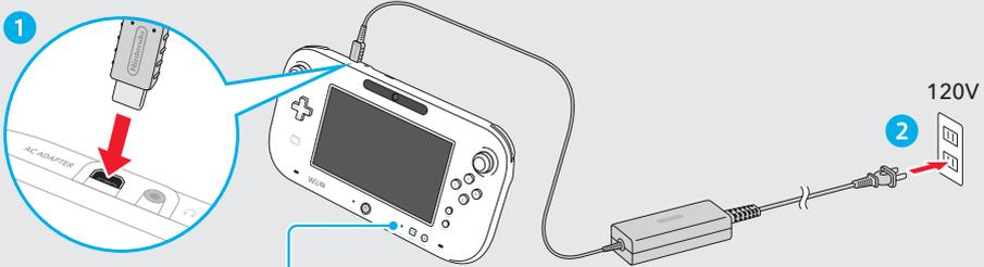
The battery LED lights up orange during charging and will turn off when the battery is fully charged.
