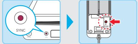
Press the SYNC Button on the Wii U console and then the SYNC Button on the Wii Remote. Follow the on-screen instructions to complete the process.
