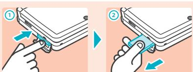
Open the SD Card slot cover and press on the end of the card until it clicks and partially ejects from the slot. Grasp the SD Card and remove from the card slot.
