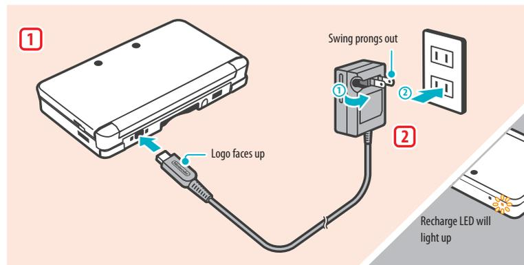
**1** Insert the DC plug from the AC adapter into the AC adapter connector on the back of the Nintendo 3DS system. Be sure to insert it straight into the connector.
