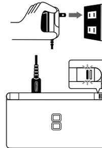
3. When fully charged, the recharge indicator LED will go out (Illustration 3). Remove the AC Adapter from the wall outlet and fold the prongs back into the housing. Remove the DC Connector Plug from the EXT Connector.
