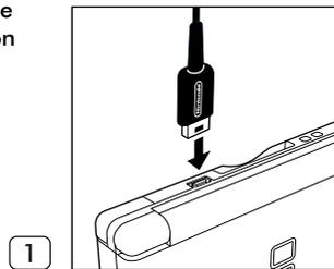
**IMPORTANT: Be sure the DC Connector Plug is facing in the correct direction before inserting into the connector to avoid damaging either the plug or connector.**
